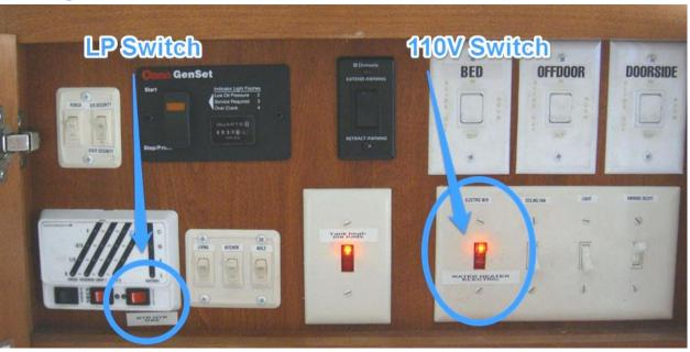
This picture is from a Landmark. Other brands will vary in what's included and where the switches are placed. In most trailers, the 110V switch is similar to a standard light switch, but lights up when turned on. The LP operation is controlled by a smaller rocker type of switch.
